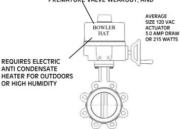
90 DEG 1/4 TURN VALVE ASSEMBLIES WITH BOWLER HAT TYPE ACTUATORS ARE NOT RECOMMENDED WHERE TIGHT & STABLE FLOW CONTROL IS
